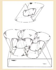
MultiConic Patent drawing: Flat surface material can be easily curved into the multiConic form. The new curved surface translates from one cone to another at the tangent line where adjacent cones touch
